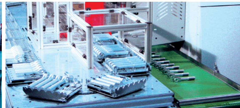
20-station pallet magazine with customer-specific pallets
