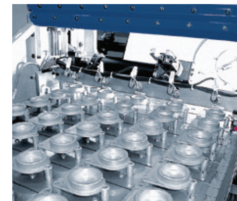
Large storage capacity chain feeding system for loading preformed blanks with the correct orientation.
