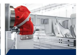
Mechanical machining of an injection mold for car bumper
