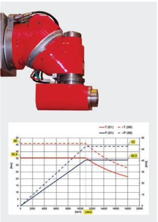
Universal milling head with automatic millesimal positioning
