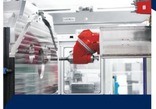
Mechanical machining of a mold by an automatic milling head 6000 rpm
